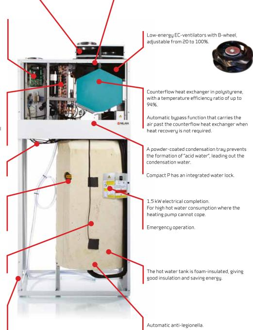
Compact P is also offered in a Polar version with a built-in preheating element to frost proof the counterflow heat exchanger and heat pump.
