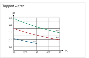
Tapped volume in liters Vmax [L] from Compact S tank as a function of tapped temperature t [C°] and tank temperature at 40°, 50° and 60°C.
