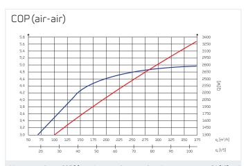
Heat output factor COP [-] supply air as a function of outdoor temperature t21 [°C] and volume flow qv [m3/h] in accordance with EN14511 at a room temperature t11 = 21°C. Blue: COP air-air / Red: Heat output supply air
