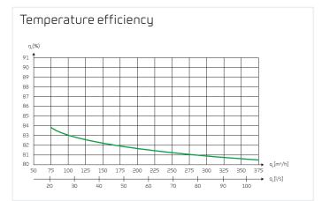
Temperature efficiency as a function of volume flow qv [m³/h] for unit with counterflow heat exchanger. Temperature efficiency acc. EN13141-7 ( $2^{\circ}$ C /  $2^{\circ}$ C). NB! The temperature efficiency, is for the heat exchanger only (without heat pump operation).
