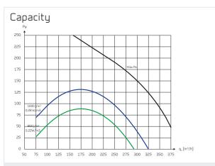
Capacity of standard unit as a function of qv and Pt, ext. Acc. EN 13141-7 for standard units with ISO Coarse >75% (G4) filters and without heating element. SEL values comprise the unit's total power comsumption.
